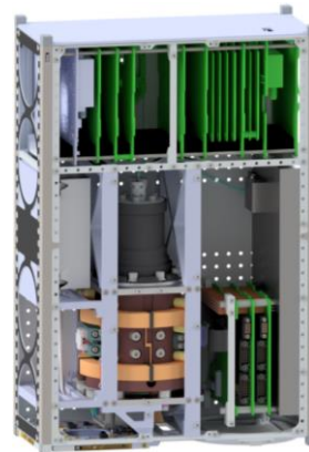
Figure 2: CAD graphic showing system architecture including Physics Package, Avionics, Laser and electronics module.
