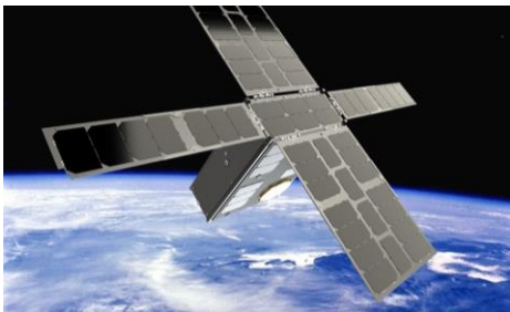
Figure 1: CAD graphic showing CASPA CubeSat during low-orbit flight. Solar panels can be seen on the system's wings to generate additional power to recharge onboard
